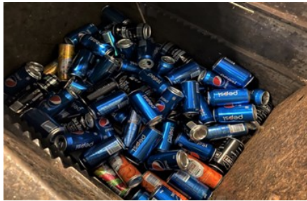
PHOTO 4: Soft Drink Cans loaded into 'The Depressor' chamber ready for crushing between the rear and front doors
