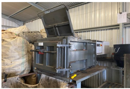
PHOTO 1: The MEC 'Depressor' – ready to be loaded with drink containers for crushing. Note the bales of crushed containers at the left side.
