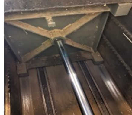
PHOTO 6: 'The Depressor' hydraulic shaft has crushed the cans between the back and rear doors
