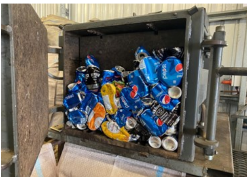
PHOTO 4: Soft Drink Cans loaded into 'The Depressor' chamber ready for crushing between the rear and front doors
