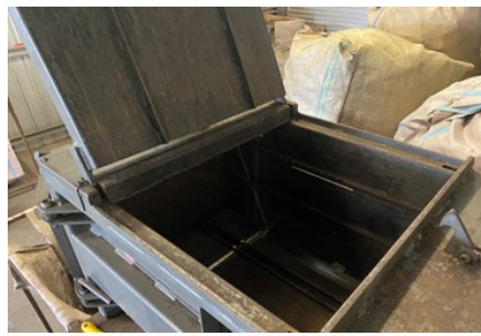
PHOTO 2: The Depressor main chamber empty with hydraulic shaft reversed to the back
