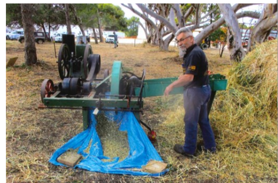
Allan McGrice cutting chaff with the Museum's 1920 Salmon Chaff Cutter and 1918 Fuller and Johnson 7HP engine
